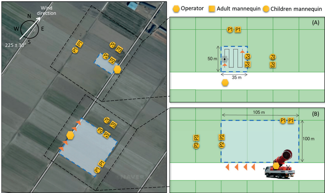
Fig. 6. Layouts of the experimental setup for human exposure assessment to pesticides using a drone sprayer (A) and a wide-area sprayer (B).
