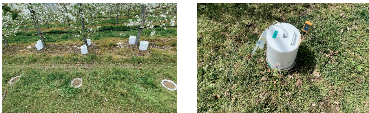
Fig. 4. Installation of closed static chambers in the inter-row space of the apple orchard for N 2 O flux measurements. Chambers were made of acrylic and consisted of a 25-cm inner diameter, a lower height of 10 cm, and an upper height of 35 cm.
