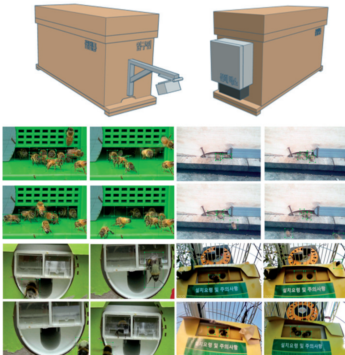
Fig. 5. Smart beehive hardware and entrance views in the experimental environments: top—schematic enclosures and sensor modules for the honey bee ( Apis mellifera ) and bumblebee ( Bombus spp.) hives; middle—example long-range entrance views for honey bee colonies at outdoor hives; bottom—example close-range entrance views for bumblebee colonies in greenhouse pollination hives.
