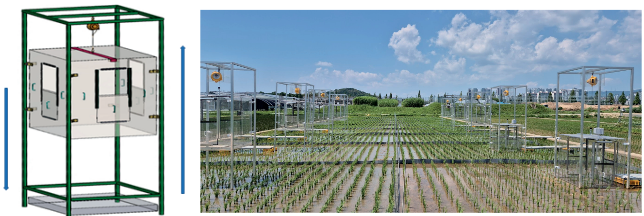
Fig. 3. Diagram of gas collection chamber for evaluation of greenhouse gas emissions in rice paddy.
